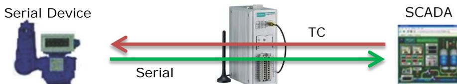
• **Transparent Serial Tunnel (TCP Client)**
